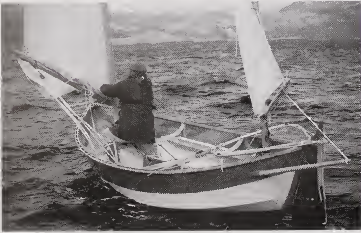
Reefing is quick when the gear is set up for it.
