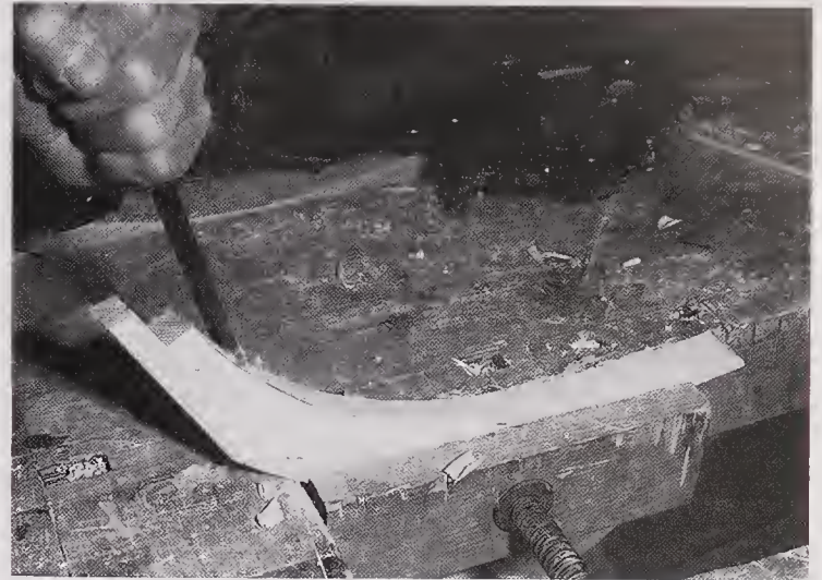
On the inside face this bevel is shaped with chisel and spokeshave.
