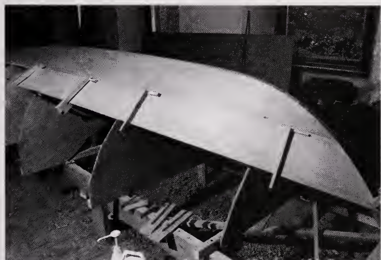
A pair of planks is cut, and the edges cleaned up and checked for fair lines.
