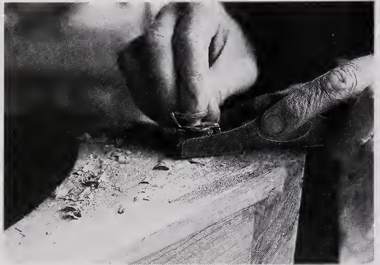
A flush stemhead is planed in line with the breasthook. The block plane is set sharp and fine to deal with the end grain.
