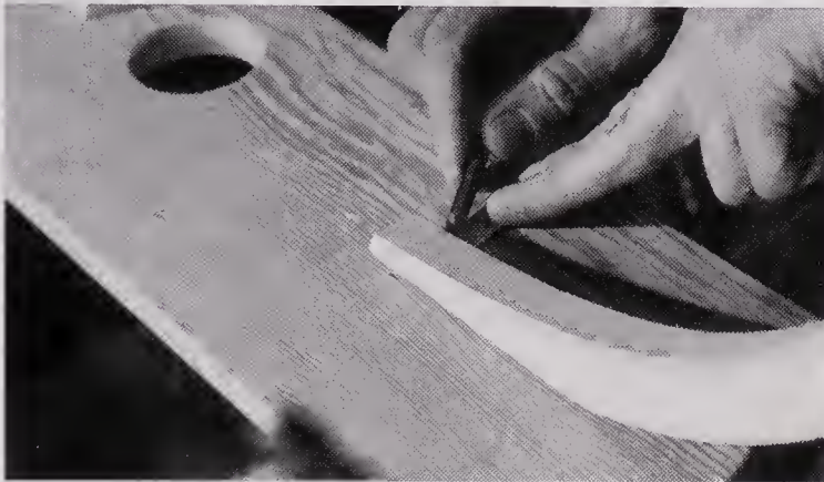
And spiled to fit the thwart and hull side.
