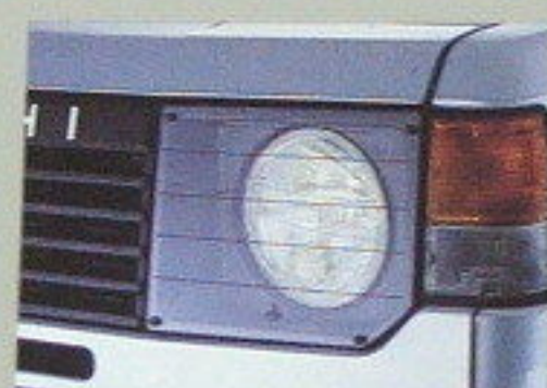
Headlamp Cover protects the glass against breakage.
